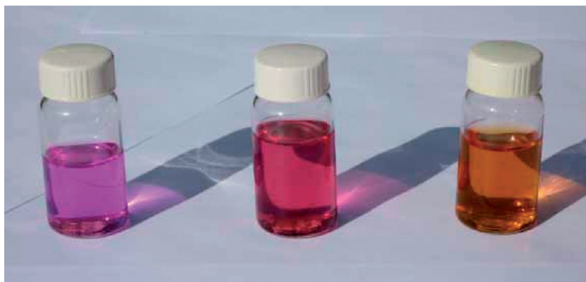
Figure 4. Photograph of dilute solutions of \text{I}_2 in (from left to right): cyclohexane, dichloromethane and water.
